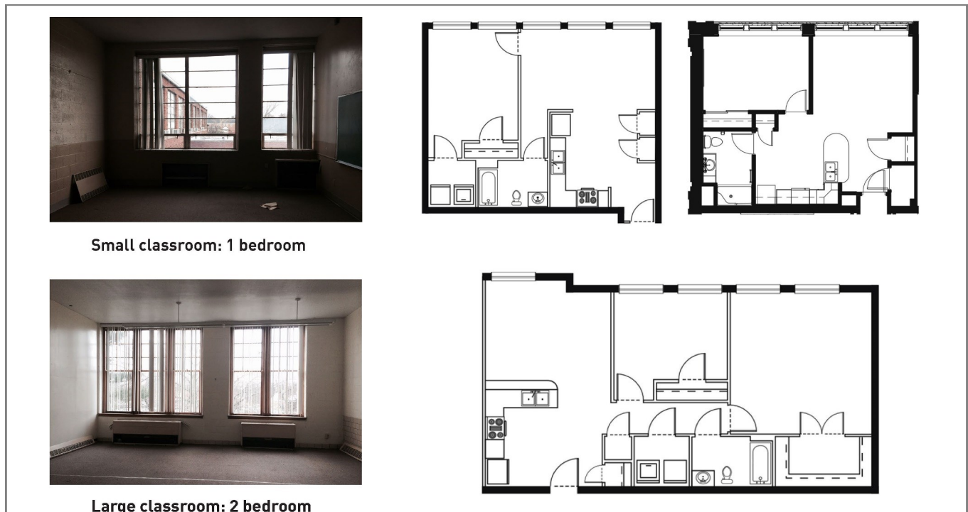
These conceptual floor plan images illustrate the possibility of transforming and repurposing a historic school into housing.
